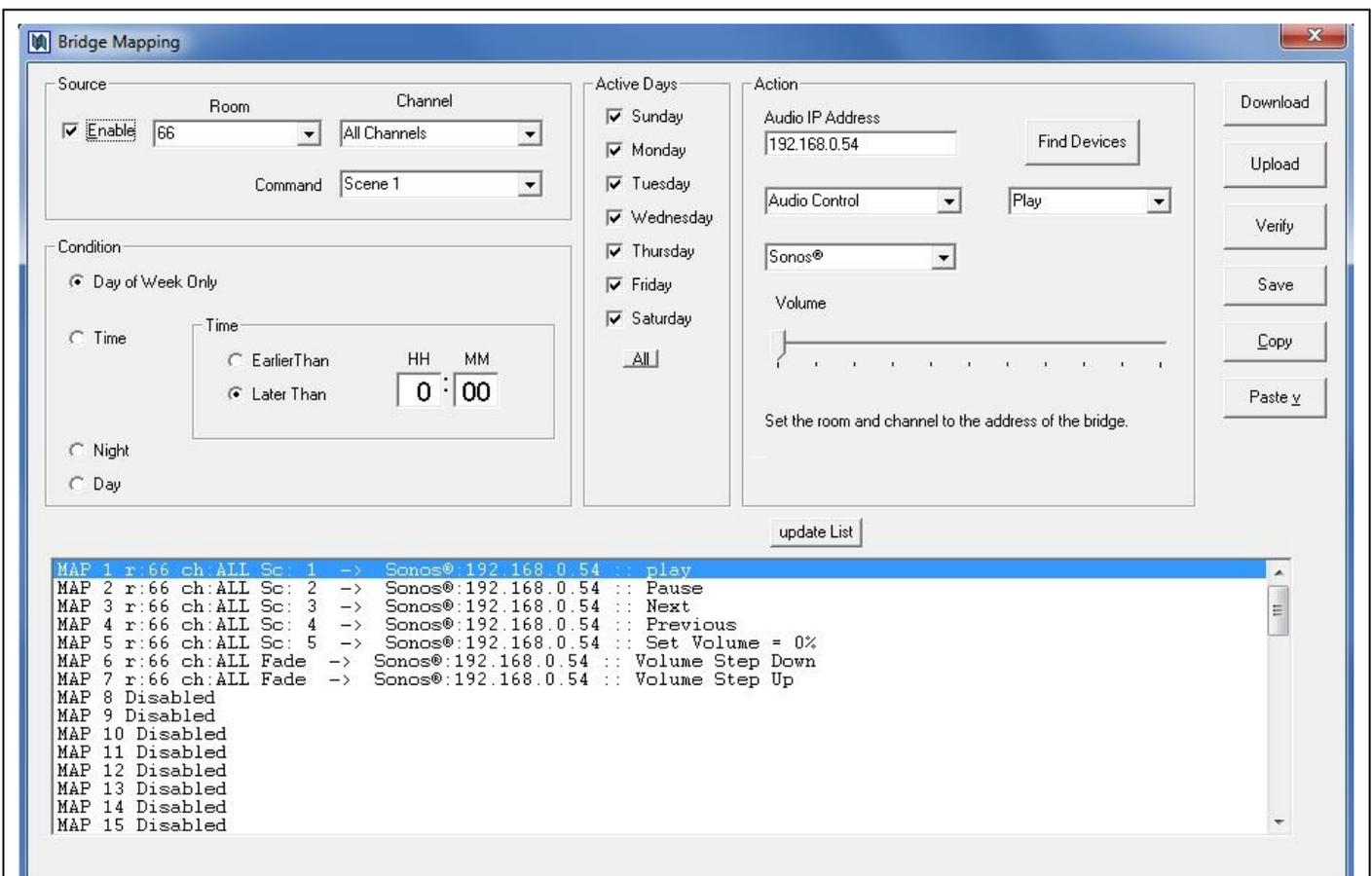
This example shows how Maps can be created within a Bridge to convert normal Scene commands to control a Sonos system
