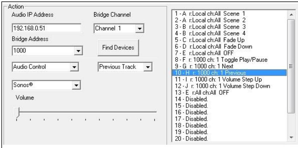
This example shows how Wired Wallplate Maps can be used to configure a wallplate to control Sonos via a Bridge fitted with ACM module
