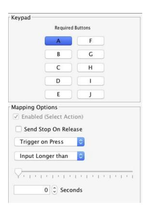
This tile defines the input to be mapped. The lettered buttons equate directly to all the buttons available for use on a RNC, often not all these will be occupied and will remain unmapped. So on a ten button plate (RNC100) all buttons A-J will be used whereas on a two button plate (RNC020) only inputs B and D are used.
