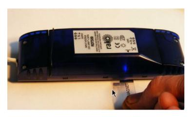
seconds until the LED starts to blink periodically showing the device is now in setup mode. Remove the magnet and the Led should continue to blink.
