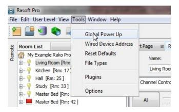
It is advised that the power up mode is either left on "off" or set to "last scene." In general it is not a good idea to have the lights come on after a power cut so a scene or percentage power up mode is best avoided unless specifically requested.
